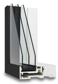
**Figure 2**: Composite window crosssection. The grey/black external profile is made from composite material and the white profile on the inside is wood. Source: Ecliptica.
