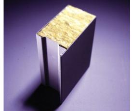
**Figure 4:** Cross-section of a steel door with a door leaf of 54 mm. The outer layer of thin steel plate encloses mineral wool insulation. Source: Daloc.
